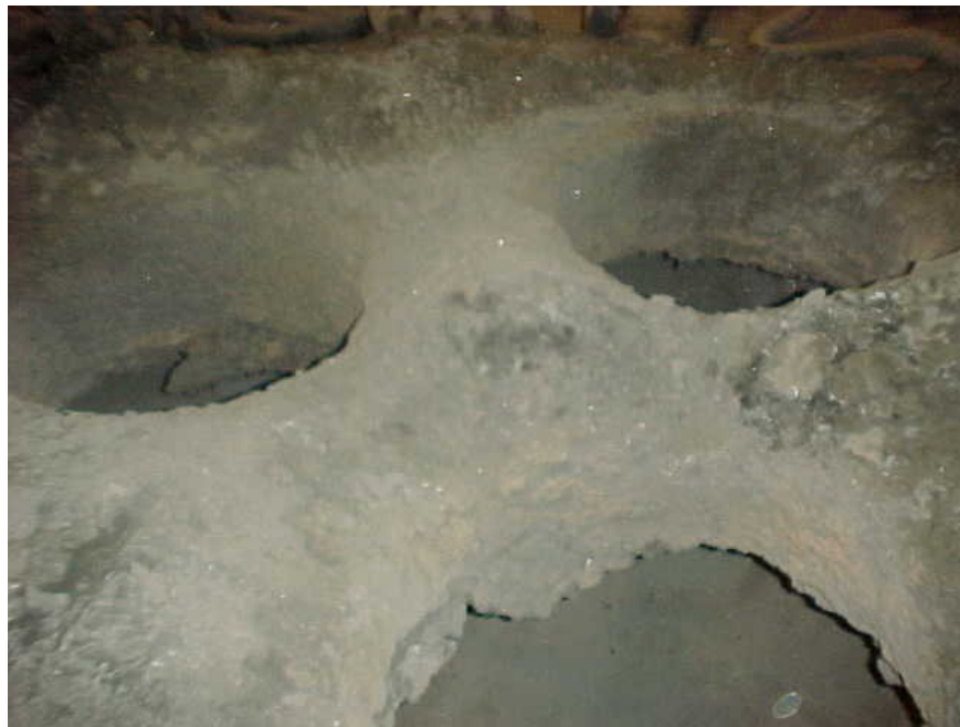
Figure 6 – Magnesium-aluminate spinel delta with high emissivity coating after 2-1/2 week's service
